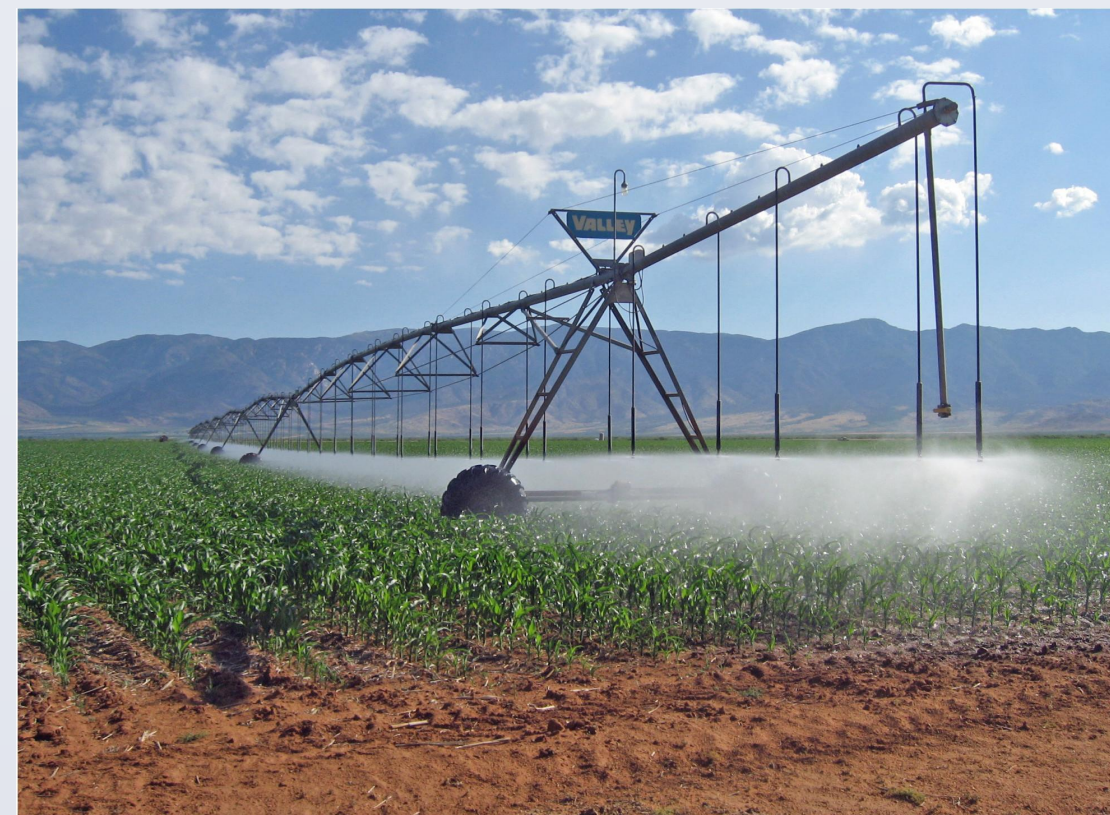
Figure 1: A center pivot irrigation system. This one does not allow for variable irrigation by regions of the field.
